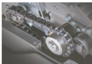
SUPER POTENTIAL POWER UNIT: chain drive system with steel gears.
